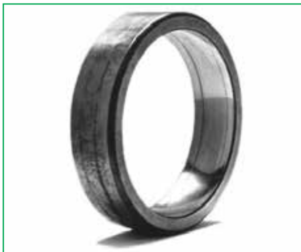
Fig. 16 Full running path pattern around entire raceway circumference of stationary outer ring of self-aligning ball bearing with rotating inner ring
